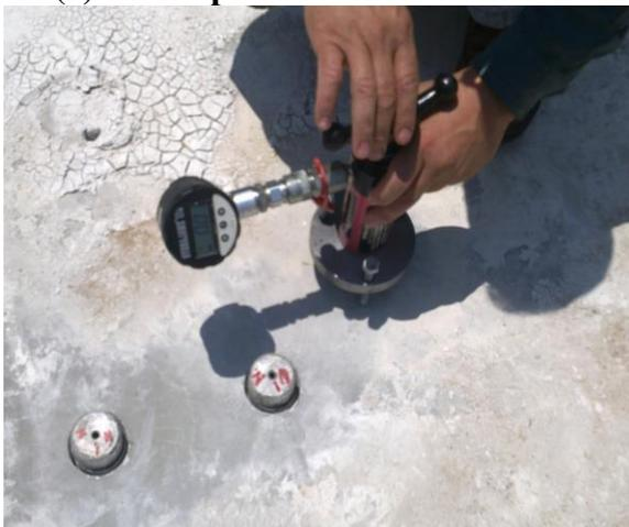
Figure (3): Pull Off test
