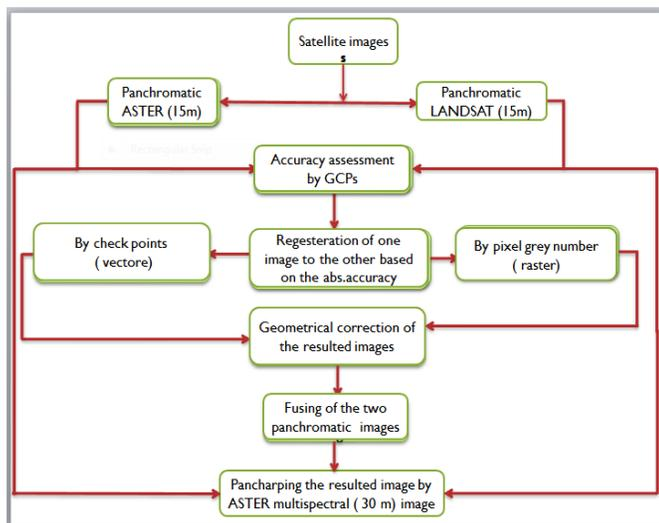
Fig.3. The methodology flowchart.
