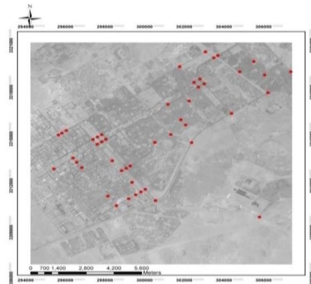
Fig. 2 .The collected GCPs over the LANDSAT image.
