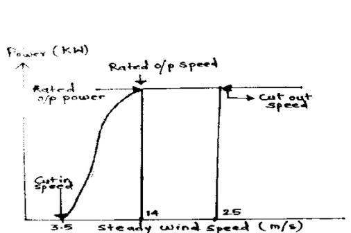
Fig.2. Typical wind turbine power O/P with wind speed.
