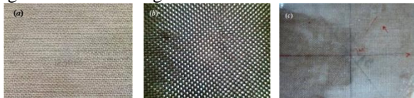
Fig. 2: Specimen samples (a) jute fiber (b) glass fiber (c) jute/glass hybrid composite (60°) fiber with 40% fiber loading
