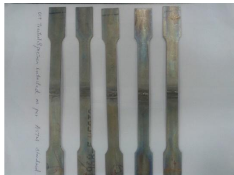
Figure 7: UIT Treatment with different pin with different speed
