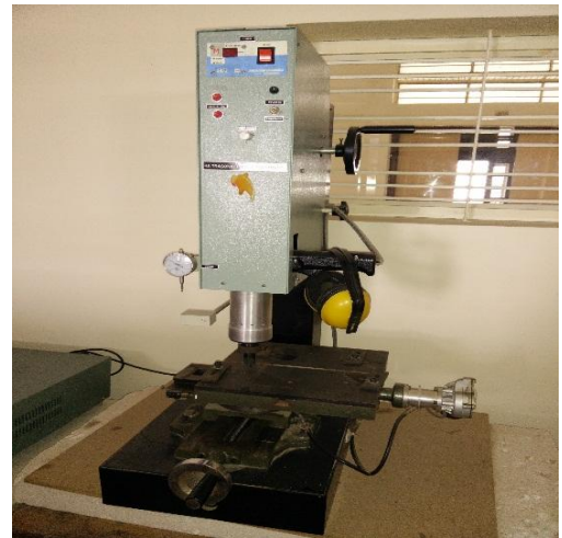
Figure 2: UIT device with fixture for automatic movement of the Impactor
