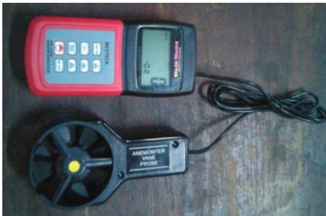
**Fig3.** Digital Anemometer
