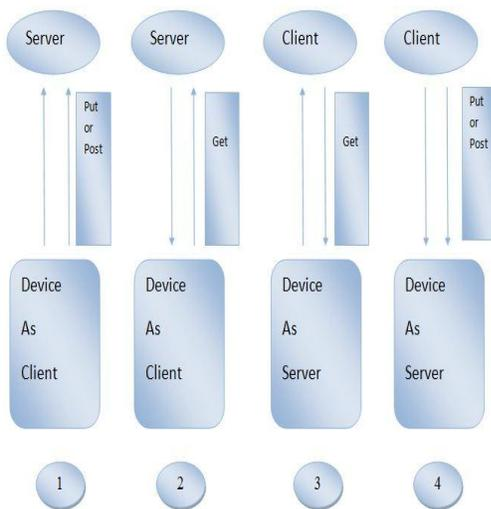
**Fig 2.5 Four ways in which device can communicate with another computer on the web**
