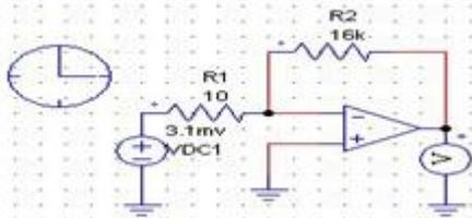
**Fig 2.4 Amplifier circuit for Geophone**
