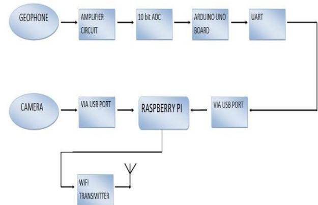
Fig 2.1 Block Diagram of Transmitter Section
