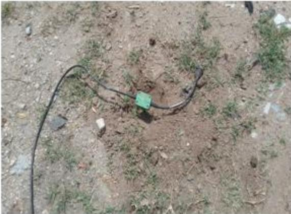
**Fig 2.3 Geophone buried in ground**
