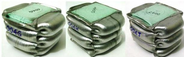
Figure 4: Crushing modes of the XPS foam filled tubes
