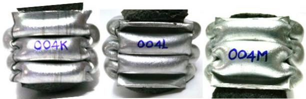
Figure 5: Crushing modes of the XPE foam filled tubes
