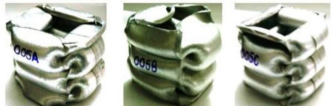
**Figure 3: Crushing modes of the empty tubes**
