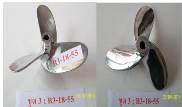
**Figure 5.** Illustration of propeller Model Type B3-18-55 (New Design, Model A)
