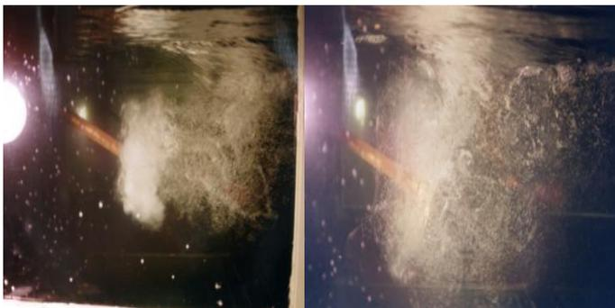
**Figure 8. (b)** Full cavitation at rotational speed 900 rpm, local
