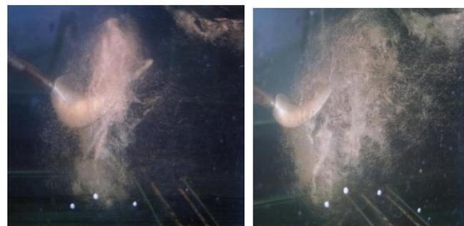
**Figure 7.** Illustration of propeller cavitation Model C at rotational speed 850 rpm
