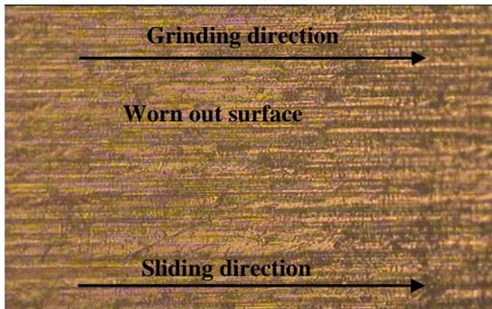
Figure 6 Photograph of the conformed block with 0° grinding direction
