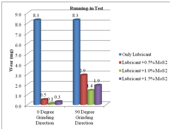
Figure 3 Initial running-in wear
