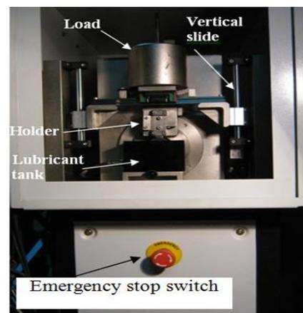
Figure 1(a) Photograph of conformal block and disk test setup [13]
