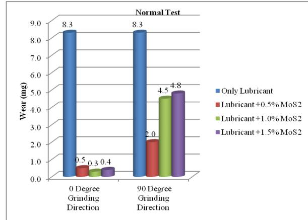
Figure 4 Wear during normal test
