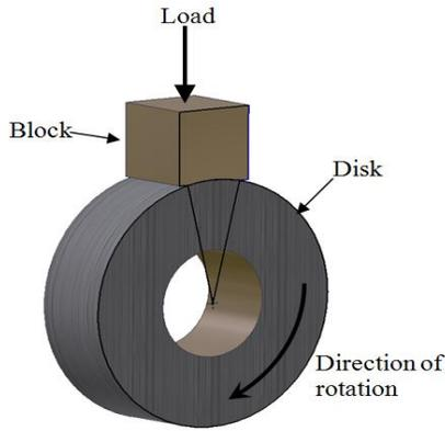
Figure 1(b) Schematic diagram [13]
