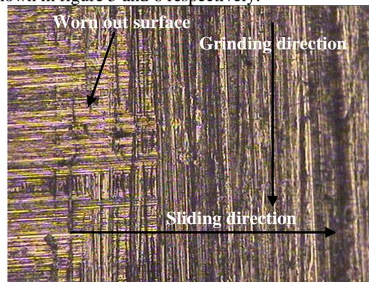
Figure 5 Photograph of the conformal block with 90° grinding direction
