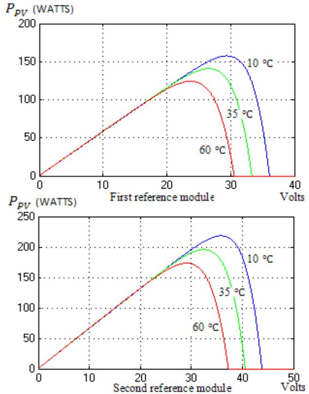
Fig. 13 P-V curves for the two reference modules at Insol. =0.7 kw/m2
