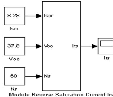
Fig. 4 Module reverse saturation current Matlab/Simulink blocks
