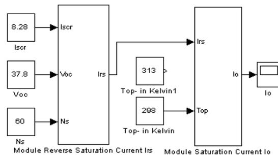
Fig. 6 Module saturation current Matlab/Simulink blocks
