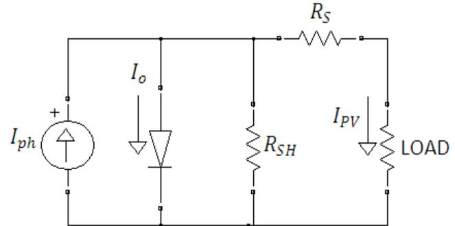
Fig. 1 PV Cell Model
