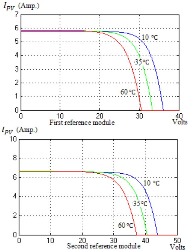
Fig. 12 I-V curves for the two reference modules at Insol. =0.7 kw/m2
