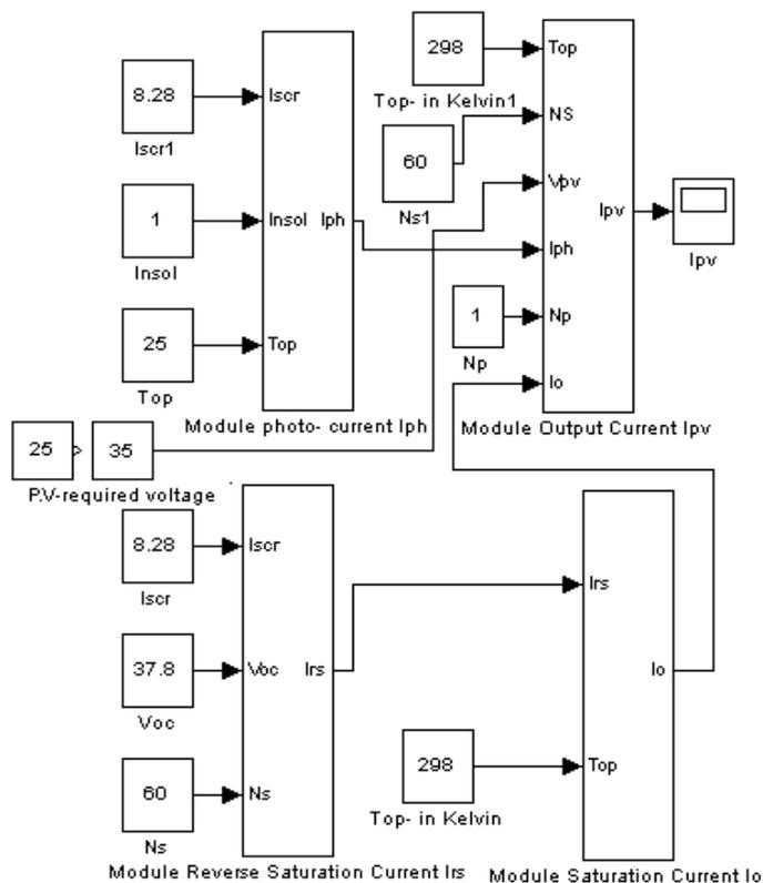
Fig. 8 Module current output Matlab/Simulink blocks
