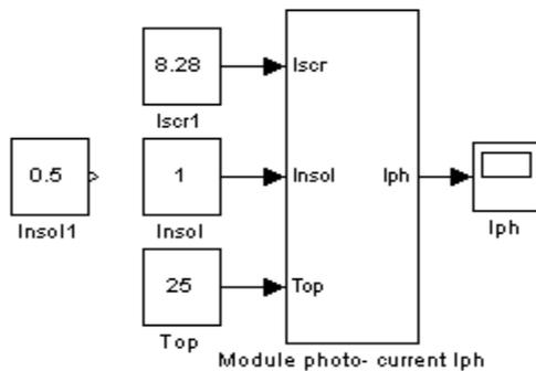
Fig. 2 Module photo current simulink blocks
