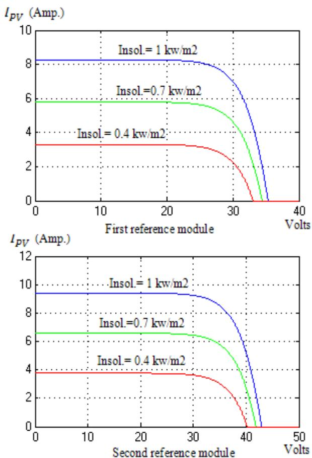
Fig. 10 I-V curves for the two reference modules at temperature =25 °C
