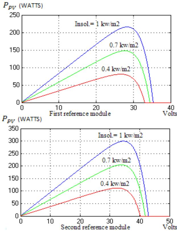
Fig. 11 P-V curves for the two reference modules at temperature =25 °C
