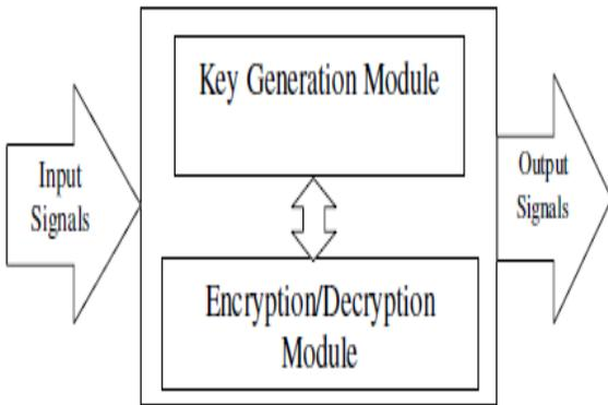
Fig. 3. AES Encryption and Decryption Unit Block Diagram
