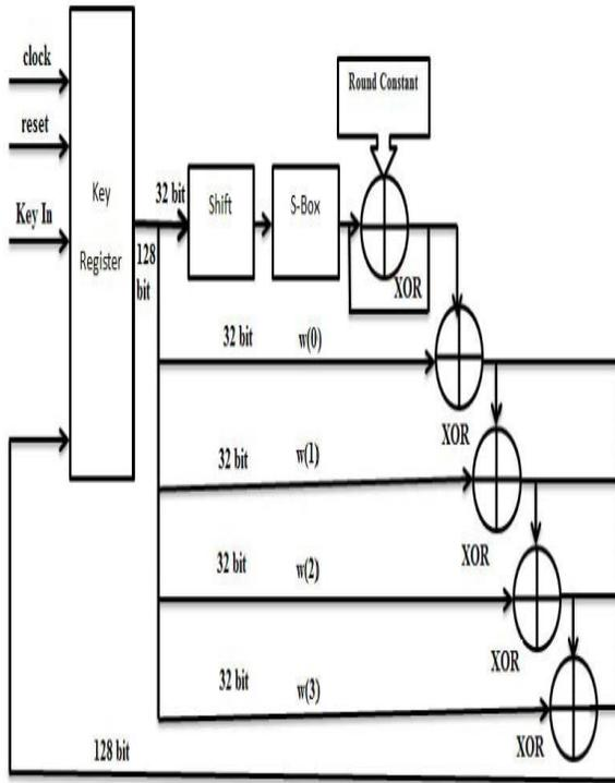
Fig. 4. Architecture of Key Generation Module.
