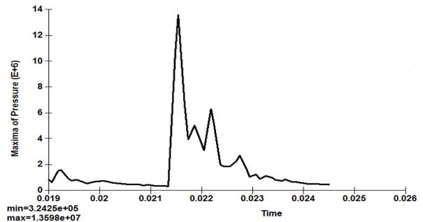
Figure (8): the maximum pressure load on concrete tank with 3750 kg TNT.
