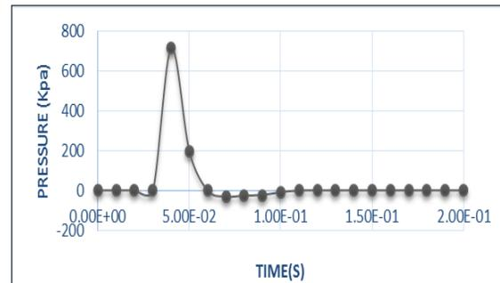
Figure (2): Pressure load on concrete block for 5000 kg through simulation and experiment.
