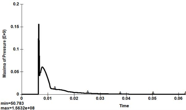
Figure (5): The maximum pressure on soil with 750 kg of TNT.
