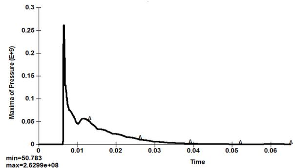
Figure (9): The maximum pressure load on soil with 3750 kg TNT.
