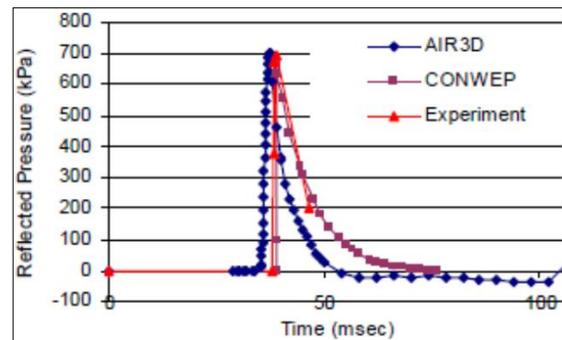
Figure (3): The accurate results of numerical and experimental methods.
