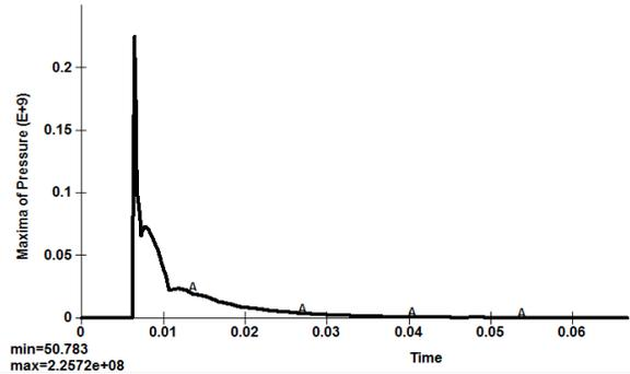
Figure (7): the maximum pressure load on soil with 1500 kg explosive material.
