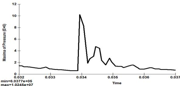
Figure (6): The maximum pressure load on concrete tank with 1500 kg TNT.
