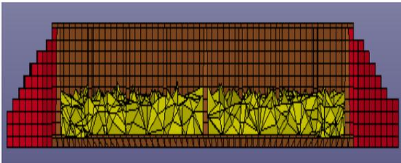
Figure (1): Numerical simulation of half buried tank.
