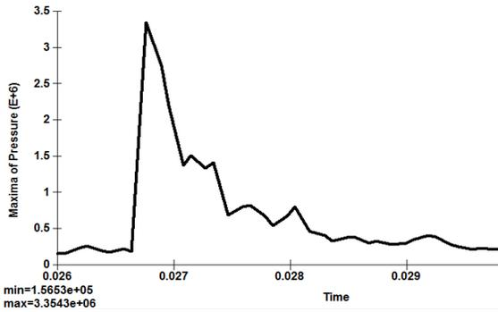
Figure (4): The maximum pressure on concrete tank with 750 kg of TNT.
