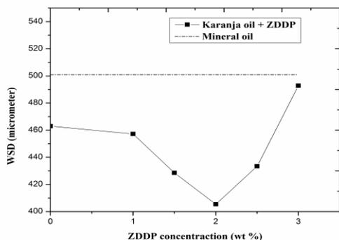
Figure 1: The relation between additive (ZDDP) concentration and wear scar diameter at standard condition.
