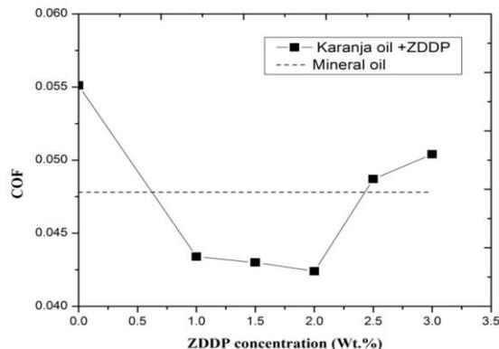
Figure 2: The relation between additive (ZDDP) concentration and coefficient of friction at standard condition.
