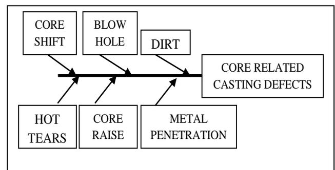
Fig.1. Fish bone diagram for core related casting defect
