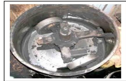
Fig.2. Muller used for mixing the sand mix
