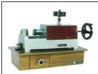
Fig.4. Universal strength testing machine
