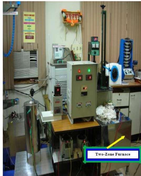
Figure (B): Proto-Type /Laboratory Furnaces (750° C & 1000° C) And Sample Lowering Facility Used For Crystallization Experiments
