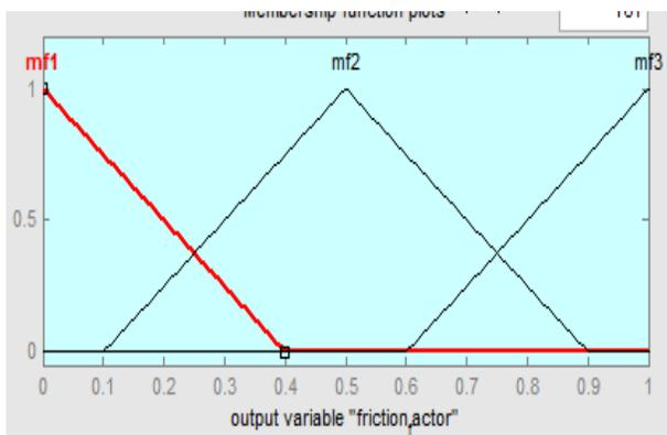
Fig-4.5. Member function for output friction factor
