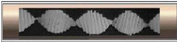
**Fig- 2:** Schematic of test tube with wavy tape inserted
