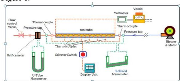
**Fig-1:** Experimental setup of Forced Convection.
