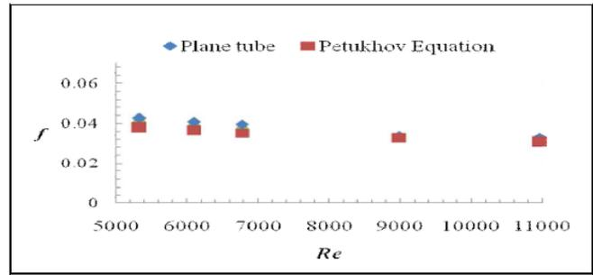
**Figure 3.1:** Validation results for friction factor
