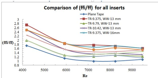
Figure 3.6: Friction factor comparison for all inserts & without insert
