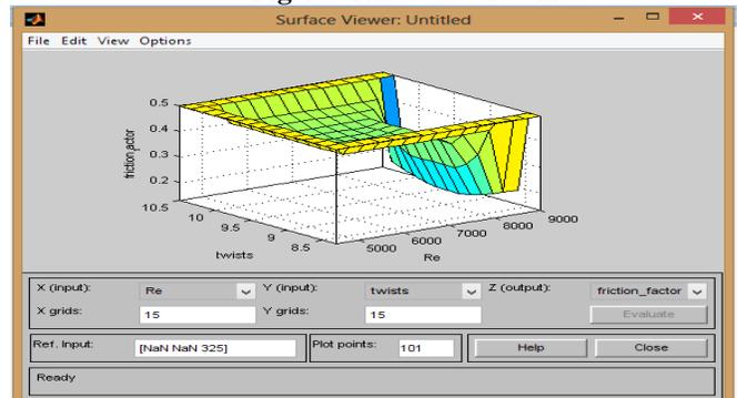
Fig. 4.9. Input Variable Reynolds number , twists and with output variable friction factor
