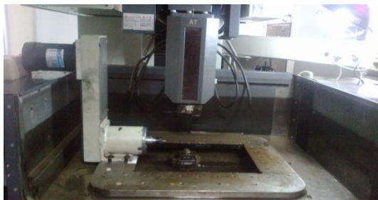
Fig 7 Developed rotary axis set up for the existing WEDM- Installed in the WEDM Machine
