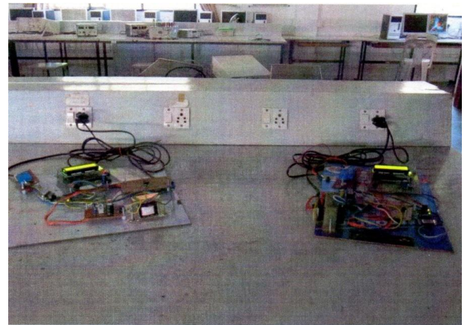
Figure 7 Experimental setup of PMUs at different locations
