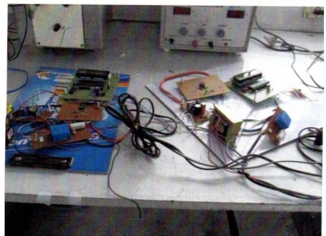
Figure 5 Experimental setup for measuring RMS values of three phase supply
