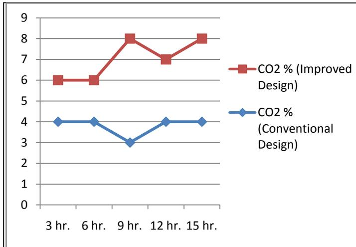
Fig.2. CO<sub>2</sub>% in exhaust gas from chimney of improved and conventional *jaggery* making plant
