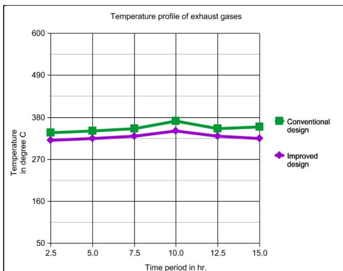
Fig.4 Temperature profile of the exhaust gases in °C from improved & conventional *jaggery* making plant
