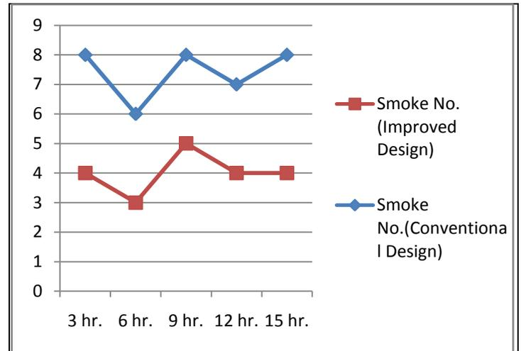
Fig.3 Smoke No. of exhaust gases of improved and conventional *jaggery* making plant
